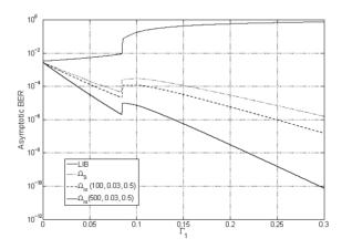
Fig. 1. Asymptotic analysis of BER versus  $\Gamma_1$  for EWF codes
